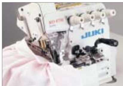
● For gathering MO-6714S-BE6-327/S162 (S162: Swing-type gathering device)
